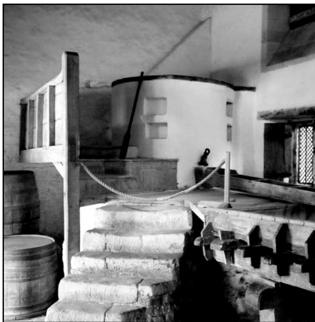
Figure 10. A private brewhouse, with copper (top) and cooler (right). This 17th-century brewhouse, in the care of the National Trust at Lacock Abbey in Wiltshire, is not on a commercial scale. The vessels would however be recognisable to the Hardys' men, for whom they represented the central core of a manufacturer's vertically integrated concern. (photograph Margaret Bird 2001)
